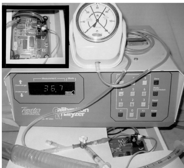
Fig. 2. Test setup used to measure intracuff pressure (CP) simultaneously with a cuff inflator and a calibration analyzer. A small, plastic T-piece was placed into the pilot line of an 8.0-mm-inner-diameter endotracheal tube (ETT) and connected directly to the pressure transducer inside the calibration analyzer (insert, upper left corner). A syringe and cuff inflator was attached to the ETT via a stopcock in the check valve at the end of the pilot tube. The ETT was placed into the trachea model.
