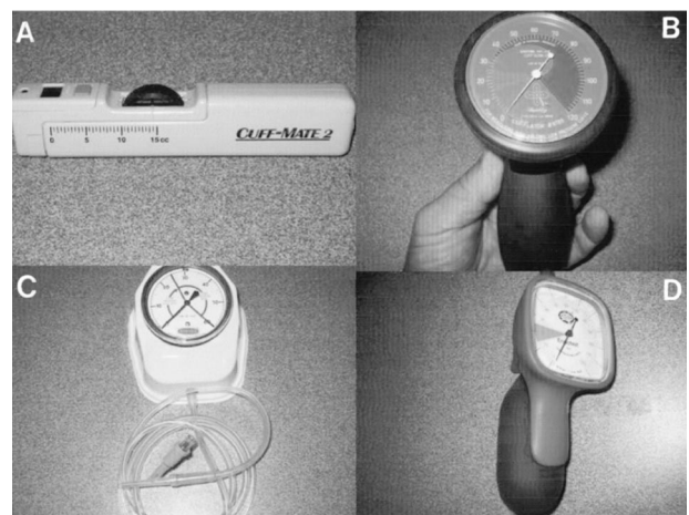
Fig. 1. Four brands of cuff inflator were tested. A: Cuff-Mate 2. B: Cufflator. C: Cuff Pressure Indicator. D: Endotest.
